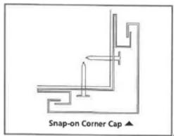
5.4.2. If the wall is taller than the Snap-On Corner Cap, notch a second Snap-On Corner Cap and lap it over on the face of the lower Snap-On Corner cap. (Image coming soon)
